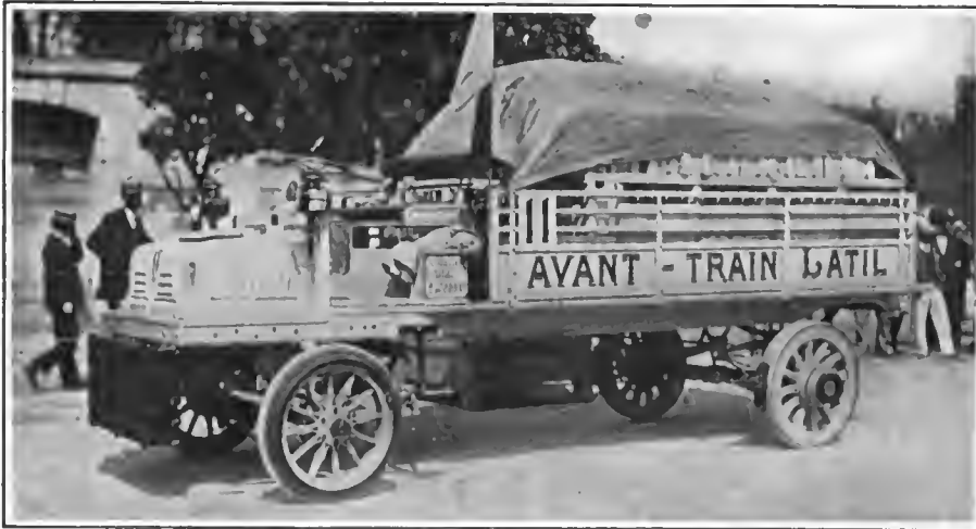
LATIL GASOLINE TRUCK IN FRENCH TRIALS WEIGHING WITH LOAD ABOUT FIVE TONS.
